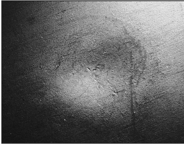
Heat sink – typical appearance on a smooth surface (1X).
