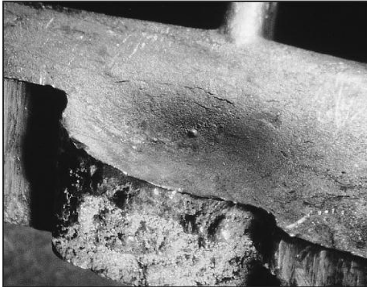
Fracture through a heat sink – the original shrink porosity under the skin is visible (7X).
