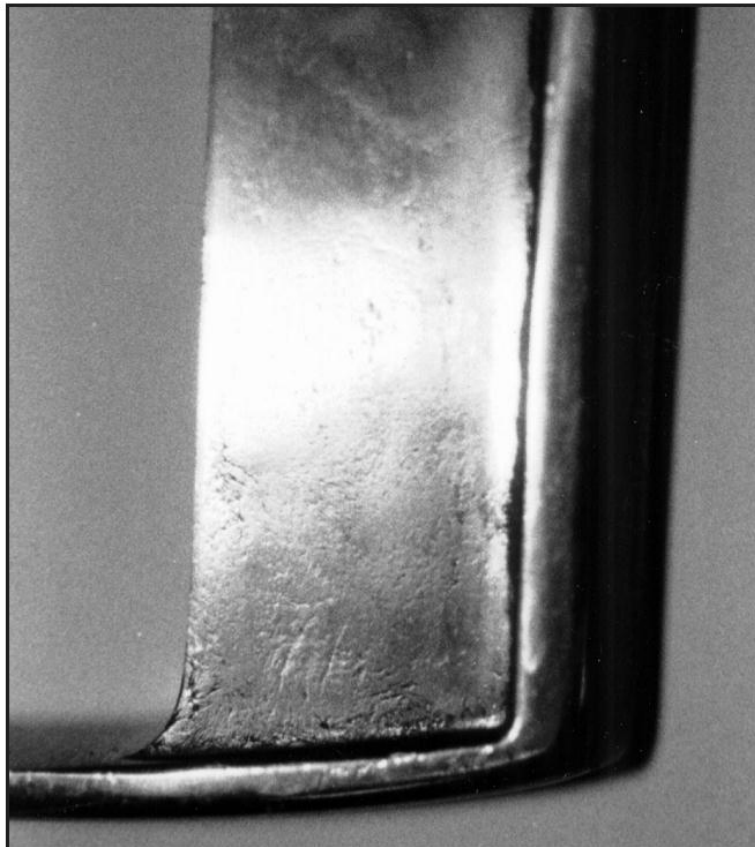
Typical surface defect (cold flow)
