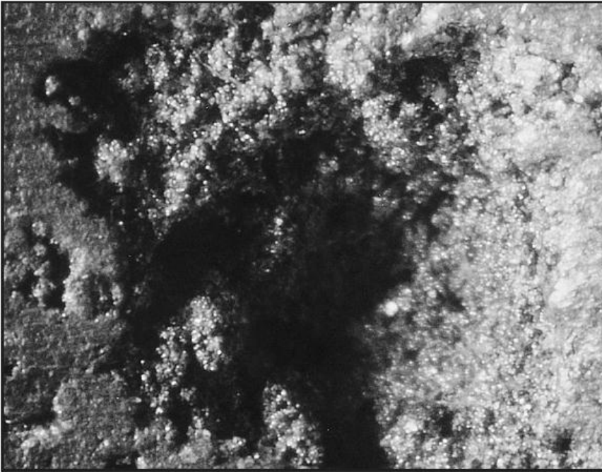
This photograph shows the rough dendritic structure on the wall of most shrink porosity (20X).
